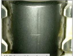
Multiple scratch marks and axial contact marks
